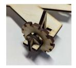
2. Place each outer wheel rim over each axle. Double check that you are using the SMALLER wheel rim without the spoke pattern. Then glue and attach the 2 other pieces as inidcated on each axle. Again, allow ample time to dry
